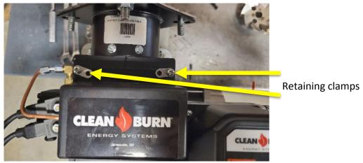
Note: Loosen screws and turn clamps to open igniter assembly.
